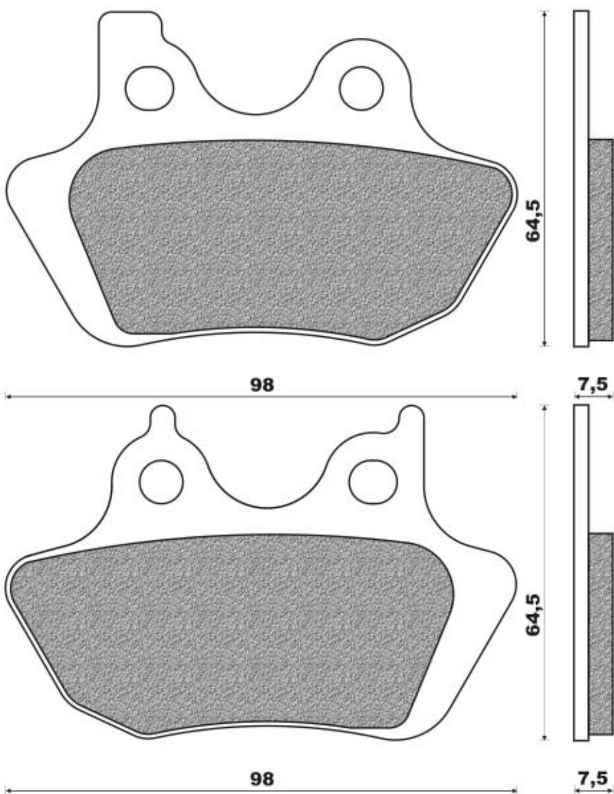
BRAKE PADS, ILLUSTRATED, BY MAKE AND MODEL | DESSINS DES PLAQUETTES PAR MARQUES ET MODÈLES
