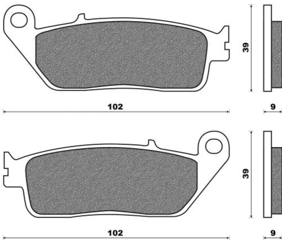
BRAKE PADS, ILLUSTRATED, BY MAKE AND MODEL | DESSINS DES PLAQUETTES PAR MARQUES ET MODÈLES
