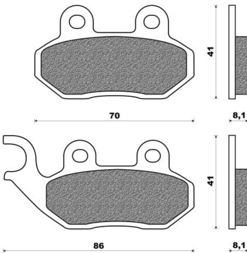
BRAKE PADS, ILLUSTRATED, BY MAKE AND MODEL | DESSINS DES PLAQUETTES PAR MARQUES ET MODÈLES
