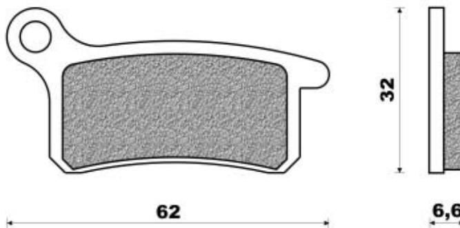
BRAKE PADS, ILLUSTRATED, BY MAKE AND MODEL | DESSINS DES PLAQUETTES PAR MARQUES ET MODÈLES
